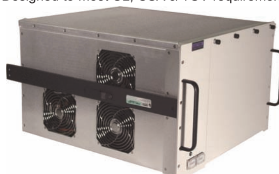
7U Model 12 Slot VME with hinged enlarged custom cover, chassis slides & 4" recessed cableway
